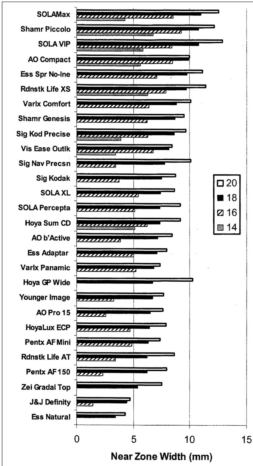
**Figure 8** Width of the near area (+1.75 D add or greater and less than 0.50 DC) at 14, 16, 18, and 20 mm below the fitting cross—sorted by width at 18 mm. Not all lenses had near zone widths at all distances below fitting cross.
