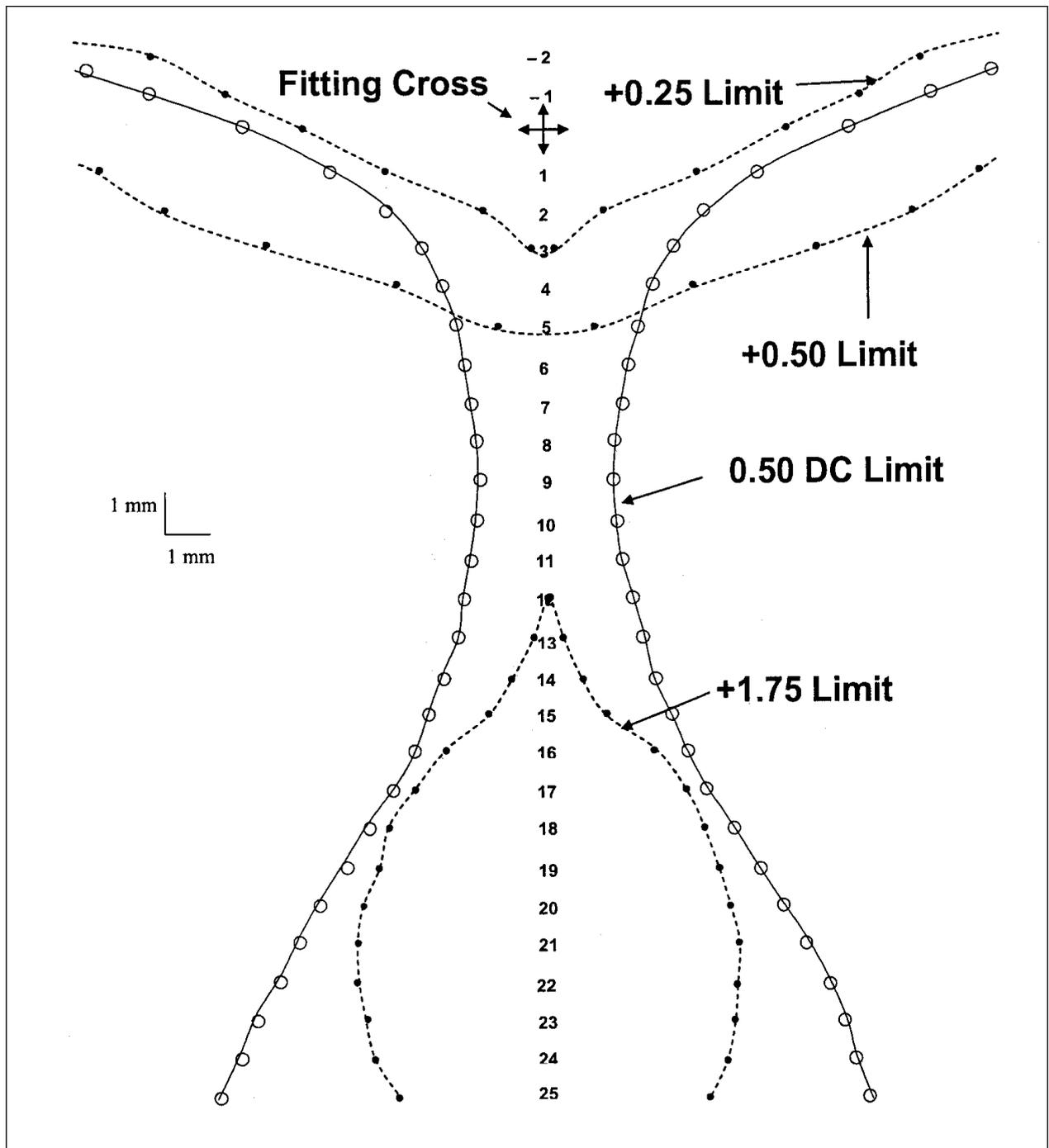
**Figure 2** Schematic diagram of selected measurements taken from the measurement data file. Measurements were taken at 1-mm vertical steps (Y value). Diagram shows typical limiting values of +0.25, +0.50, +1.75, and 0.50 DC.
