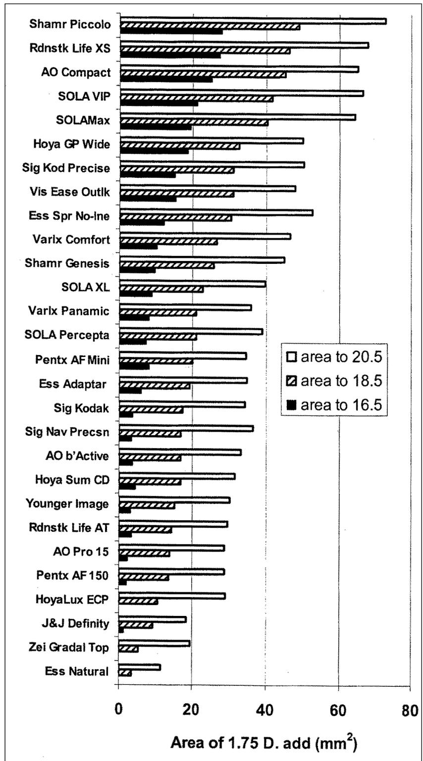
**Figure 9** Cumulative area of the +1.75 D add (mm<sup>2</sup>) to 16.5, 18.5, and 20.5 mm from the fitting cross—sorted by cumulative area to 18.5 m from fitting cross. Not all lenses had cumulative areas corresponding to the measured distances below the fitting cross.
