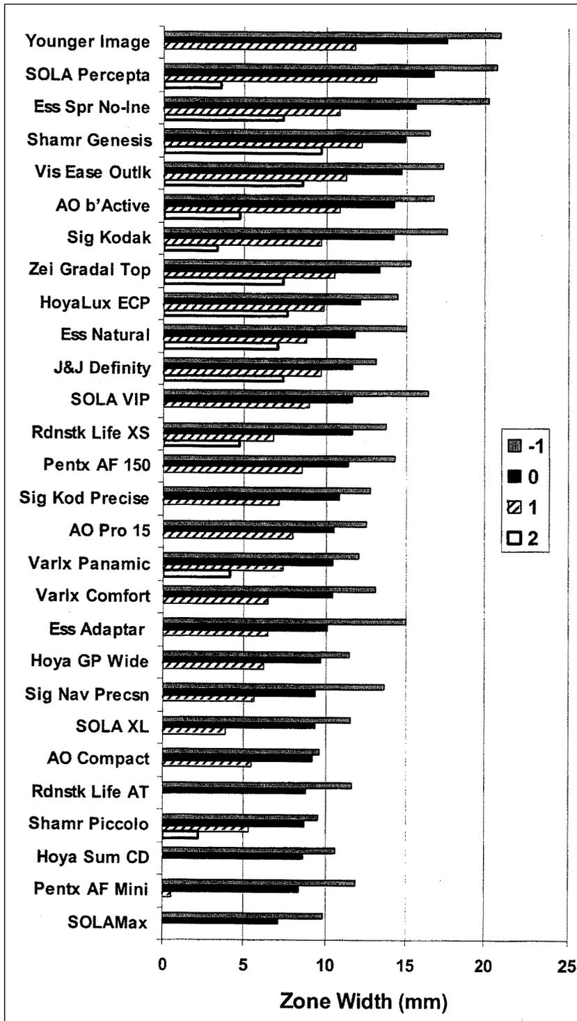
**Figure 3** Width of the distance power (within  $\pm 0.25$  DS and less than 0.50 DC) at fitting cross (0), above (-1 mm), and below (1 and 2 mm) the fitting cross. Not all lenses had distance area at 1 and 2 mm below fitting cross. Lenses sorted by width at fitting cross.
