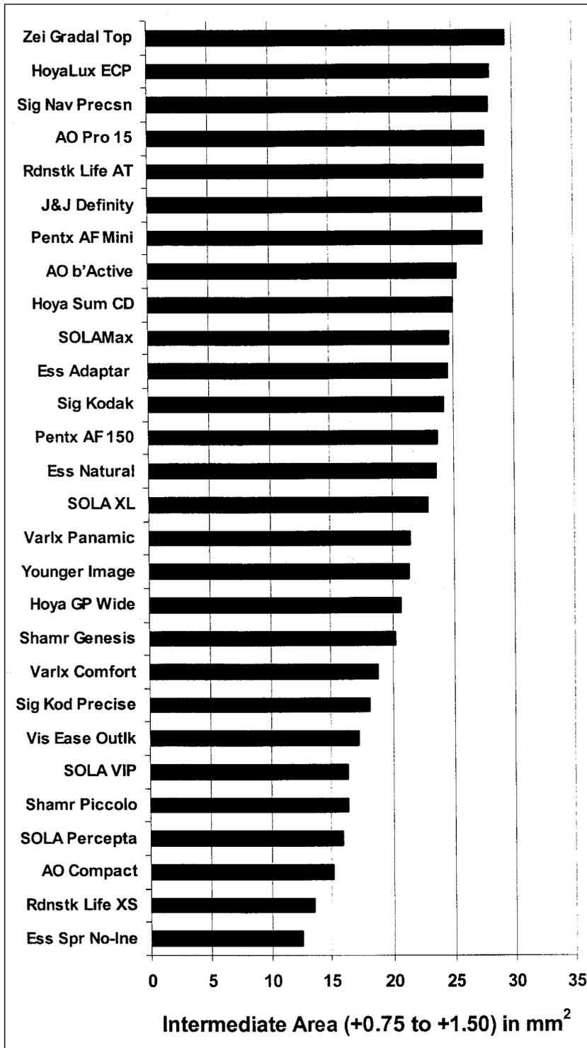
**Figure 6** Area of intermediate power (+0.75 to +1.50 add and less than 0.50 DC) in mm<sup>2</sup>.
