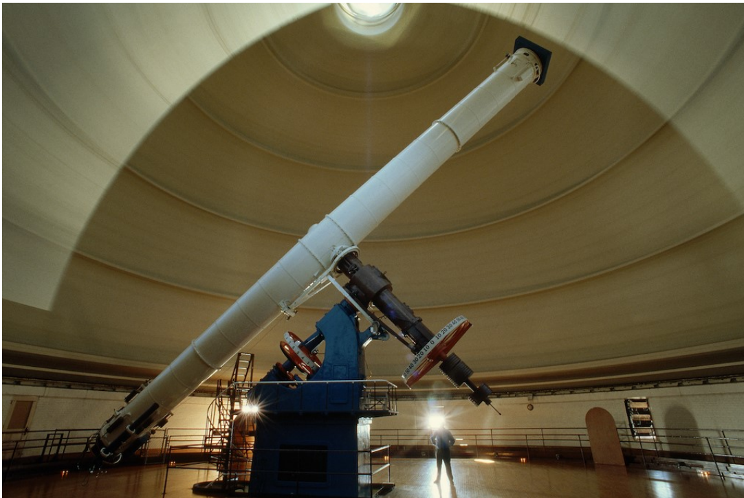
Fig. 15. The 40" refracting telescope at the Yerkes Observatory. The lens was made by Alvan Clark & Sons, the tube and mounting by Warner & Swasey Co. of Cleveland. It remains the largest operating refracting telescope in the world. The focal length of the lens was 63 feet, so the tube had to be at least that long.
